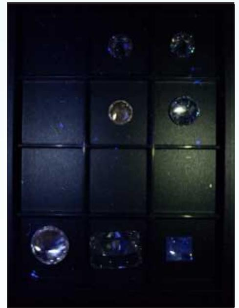
Only the natural diamond on the bottom right shows some blue fluorescence. Simulants and lab grown diamond will never show fluorescence under Long UV illumination.
