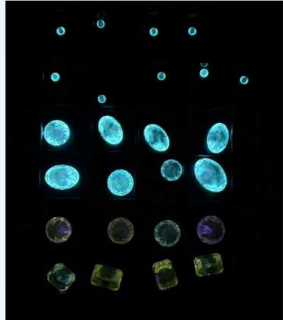
HPHT lab grown diamonds show blue fluorescence but will be painted in red due to their phosphorescence.
