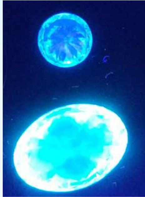
The HPHT lab grown diamonds and NATURAL diamonds fluoresce in blue. However, due to the fact that HPHT lab grown diamonds show phosphorescence, it will be marked in red in the **RESULT** picture.
