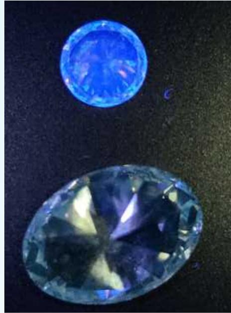
Under Long UV illumination, the oval (which is an HPHT lab grown diamond) does not show any fluorescence. Some of the natural diamonds show fluorescence.
